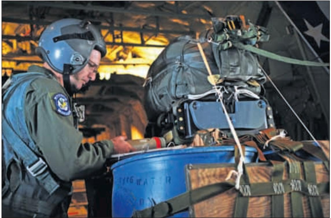
Master Sgt. Jason Beebe, 37th Airlift Squadron loadmaster, prepares the Joint Precision Airdrop System bundle for the first test employment during a joint training mission in Europe Oct. 23 at Powidz Air Transport Base, Poland. The JPADS is equipped with a GPS, allowing the bundles to land within feet of the point of impact, ensuring they get to war fighters.
